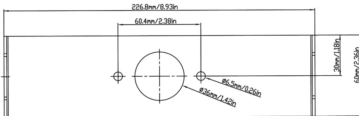
Figure 2-8 Dimensions du support de montage i-DT33XW
