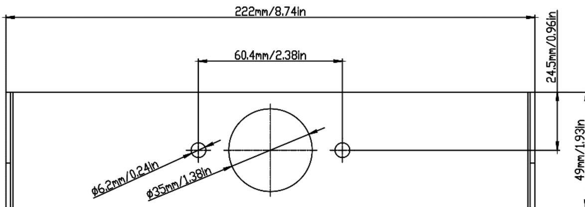
Figure 2-7 Dimensions du support de montage i-DT33P
